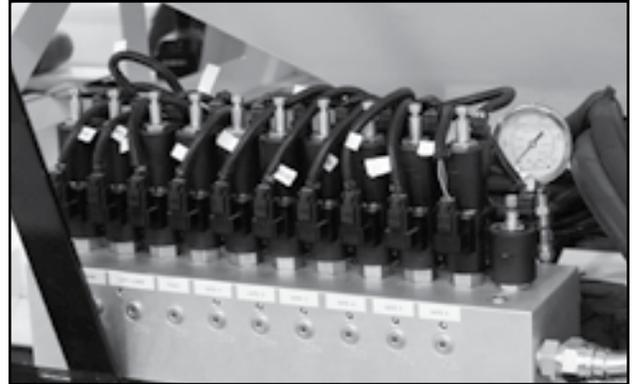
Fig 39 - Hydraulic valve block
