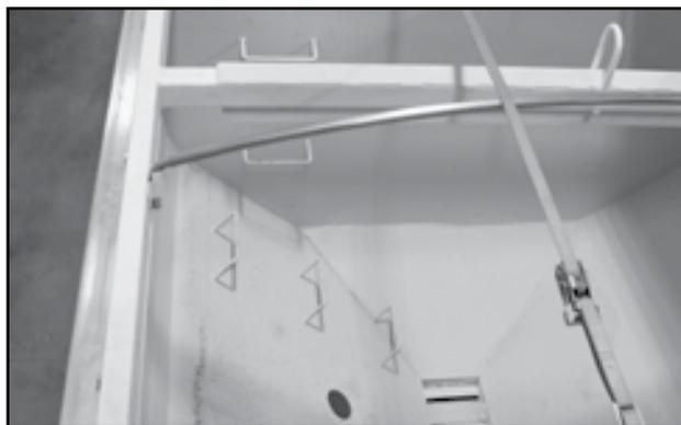
Fig 22 - Compartment ladder rungs
