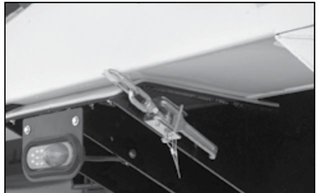
Fig 41 - Rear conveyor latch
