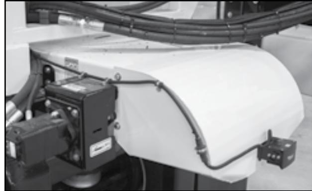
Fig 60 - Slave conveyor discharge hood
