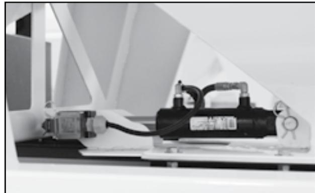
Fig 37 - Compartment gate cylinder
