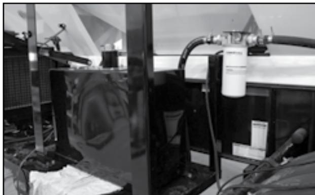
Fig 64 - Hydraulic reservoir and filter
