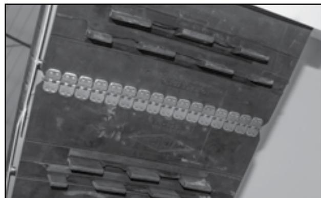
Fig 63 - Alligator lacing on rear conveyor paddle belt
