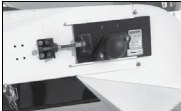
Fig 57 - Adjustment bolts on rear conveyor
