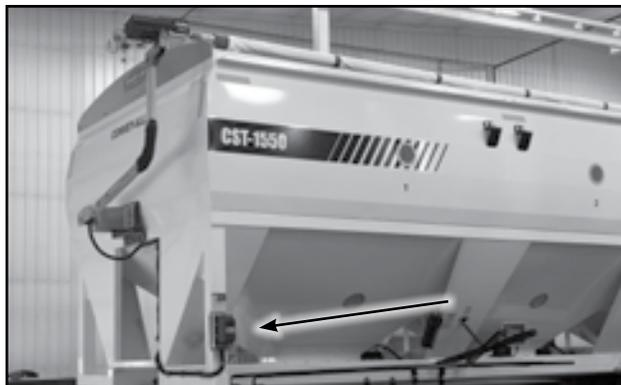
Fig 21 - Roll-top tarp controls
