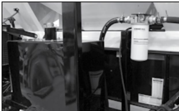
Fig 53 - Hydraulic system oil filter
