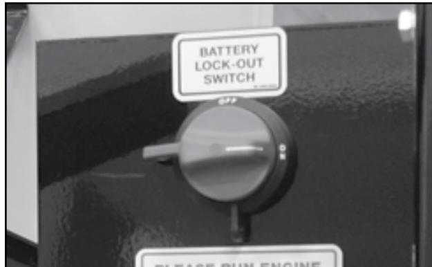
Fig 31 - Battery Lock-out
