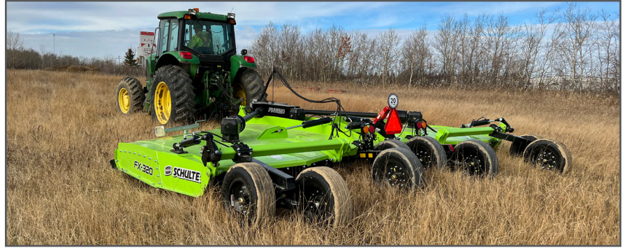
Available with walking axles as shown or straight through axles
