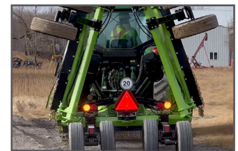
Narrow 106" transport width and over-centering wing design
