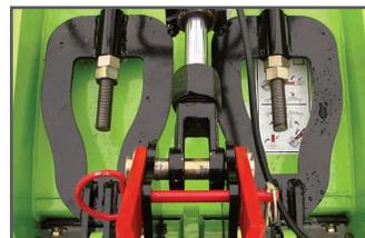
Dual levelling rods with floating hitch
