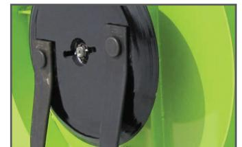
7 gauge spun formed stump jumper pans
