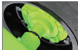
Metal seal guards on 517 hubs
