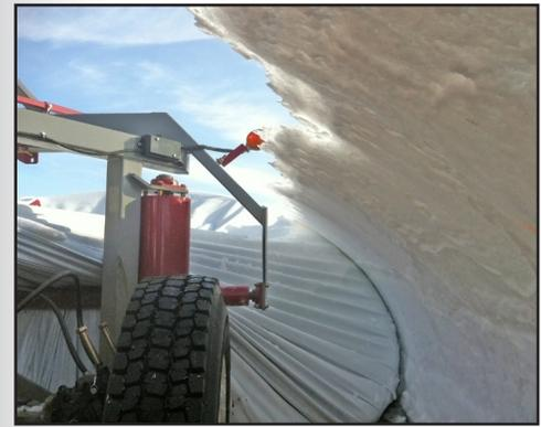
Pictured above is a GrainBoss working in a grain bag banked with snow. The narrow roller design eliminated need for extensive snow removal.
