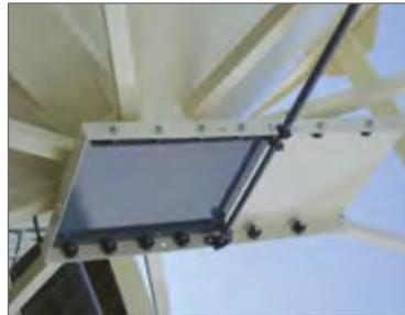
**Rack-n-Pinion slide gate assembly**
