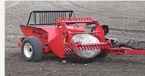
By positioning the rake and using the reels as a support, the RR250ST can pick rocks up to 24" x 45" (61 x 144 cm) and the RR900ST picks rocks up to 28" x 55" (81 x 140 cm).
