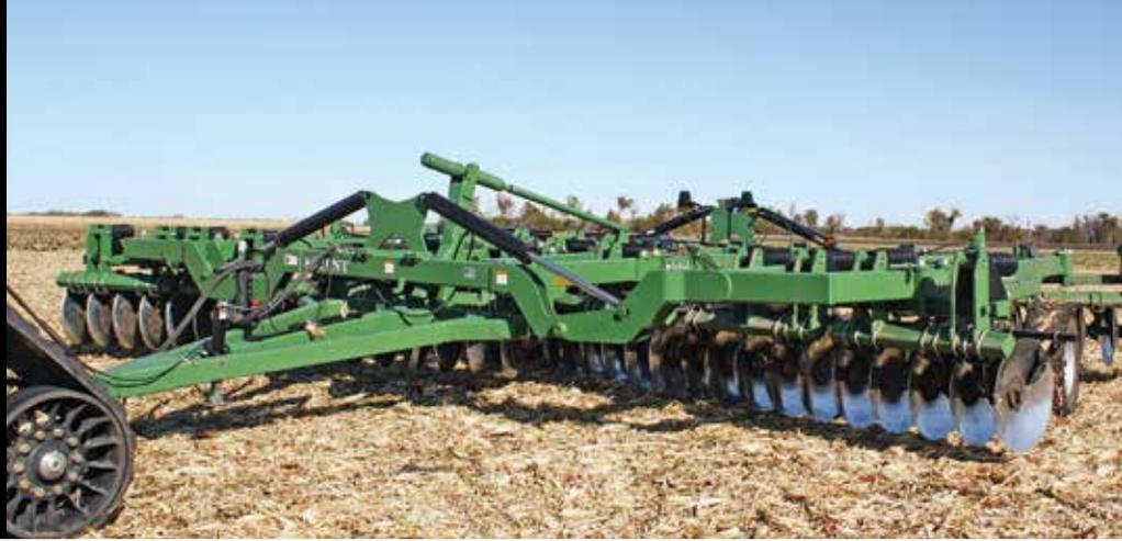
The Wishek Tandem Disc is the industry's workhorse when it comes to heavy-duty discs. Wishek discs are manufactured to an industry-recognized level of performance that separates them from the competition. Wishek discs give you a powerful tool utilizing their rock cushion and 22.5 truck tires.
