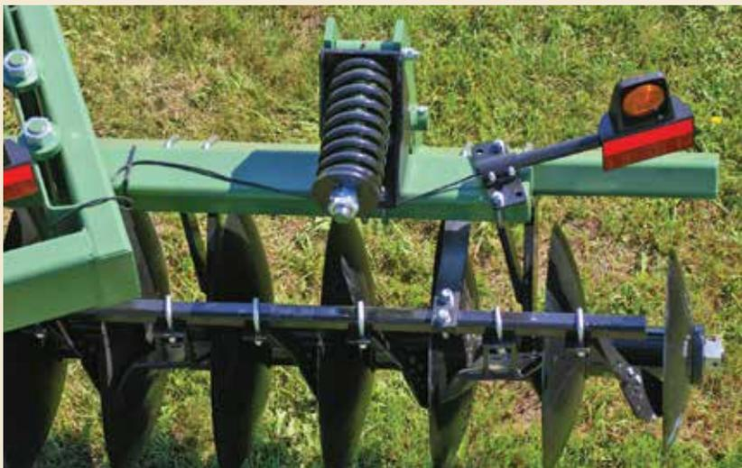
Spring cushion models of the Wishek Tandem Disc offer unique flexibility in their design. When a blade strikes a solid object, it travels in an arc of 12 inches (305 mm) rearward and upward, letting it travel over and avoid damage from impact with that object.
