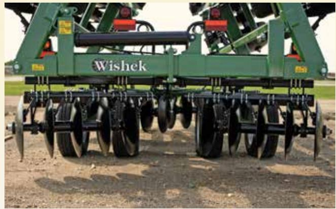
With strength designed in every machine, Wishek disc harrows are heavy-duty machines that have the heaviest weight-per-blade specifications in the industry. This allows Wishek disc harrows to work in almost all soil conditions and crop residue. Disc gangs are set at an angle in order to mix residue regardless of field and residue conditions with just the right amount of soil to help create an ideal seed bed.
