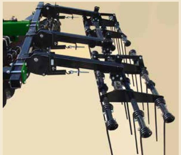
To assist in leveling the field and help create a better seedbed, add a 3-bar harrow. The tubular tooth bar harrow features  $\frac{5}{16}$  x 26-inch-long tines (16 x 660 mm) for strength and durability.
