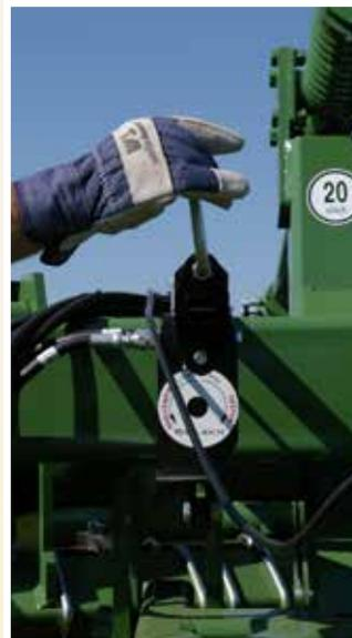
Single-point depth control allows the operating depth of the entire disc to be adjusted with a single setting. This simple adjustment, done at the front of the machine, is easy, safe, and precise. Single-point depth control is optional on all models.
