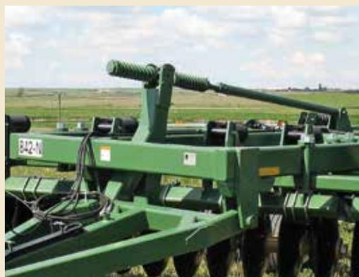
Standard adjustable leveling system levels the unit front to rear. A hydraulic leveler is optional.
