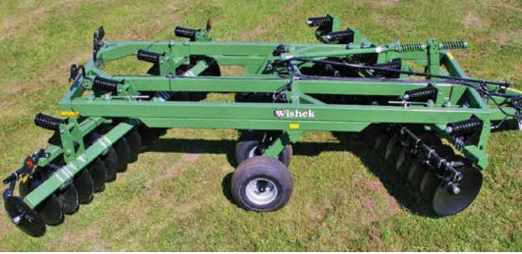
The Wishek Offset Disc is for those customers seeking the time-tested, proven design of an offset disc, coupled with Wishek's reputation for building strong, heavy-duty discs. Wishek discs are the most reliable and lowest maintenance discs on the market. With nearly 1,000 pounds per foot (1,488 kg/m), the Wishek Offset Disc has the brute strength to penetrate in even the most demanding soil conditions.
